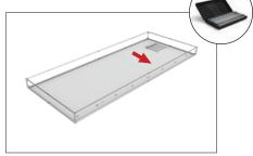
**Step 14: Turn. Position. Lock.** Insert tensioning pole into the bottom of display. Keep the pole flat until the entire pole fits inside the frame. **Turn** the pole 45°. **Position** and
