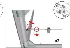
**Step 7:** Continue inserting silicone edge of graphic into the frame working towards the center of frame on each side. Do not over pull or stretch.
