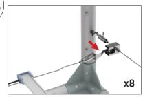
push pole onto the red indicators at top of frame. **Lock** the bottom of the pole by firmly sliding or knocking the the pole into place over red indicators
