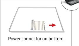
**Step 3:** Attach each LED Light Array to top and bottom of frame.
