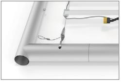
Step 2: Take out the LED Lights and gently unroll on the ground with lights face down. WARNING! Do not drag lights across ground or it could break the LED lights.
