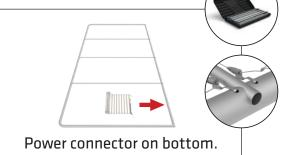
**Step 3:** Attach each LED Light Array to top and bottom of frame.
