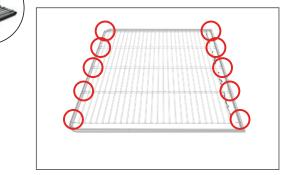
Pull extra cable leash at bottom to secure each LED Light Array into place.
