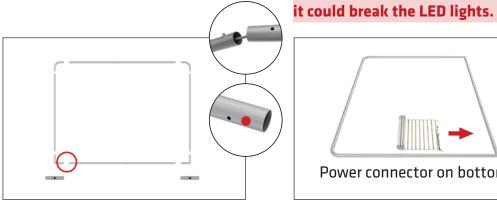
Step 2: Take out the LED Lights and gently unroll on the ground with lights face down. WARNING! Do not drag lights across ground or
