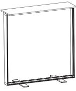
Install graphics by pressing silicone edge into channels
