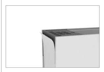
**OPTIONAL:** Connect frames together using u-clamp to create a continuous wall.
